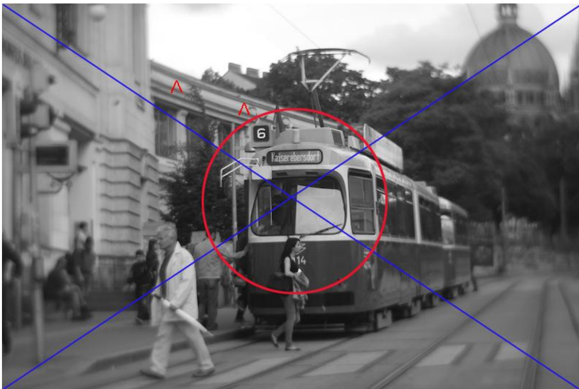
Figure A –Modern photograph using Petzval lens. The red circle depicts the area of focus of the Petzval lens (Note the clarity); the X depicts the center of the picture, and the red carets highlight where the pincushion effect is observed (the bow in the wall line.) Notice how defocus increases and brightness decreases radially outward from the red circle (see people on steps and the dome in the background.) See http://www.strongmocha.com
